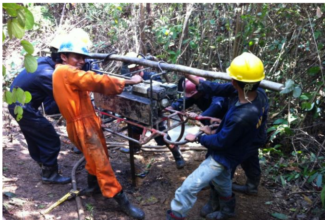
Shot-hole Drilling Operations on SBA Seismic Survey
